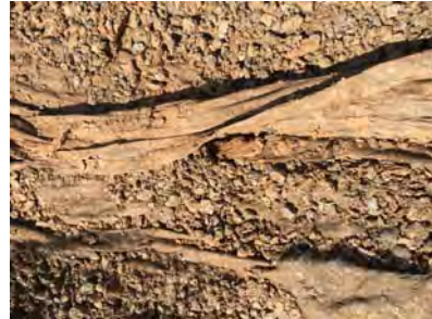
Silted over non-woven filter fabric
