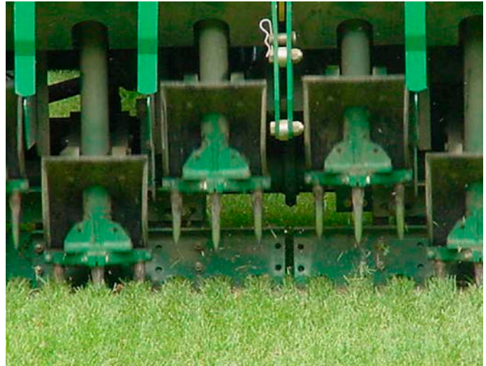
Aerification with solid tines is a great way to improve conditions during the season because it causes minimal surface disruption but it should not be used as a substitute for hollow-tine aerification.
