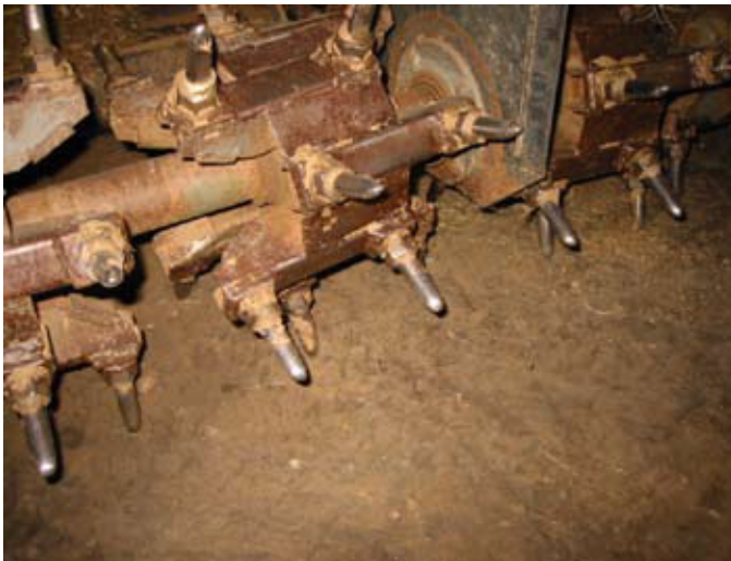
Figure 2. Using solid tines like these to aerify can help increase water infiltration and oxygen levels in the rootzone with little surface disruption
