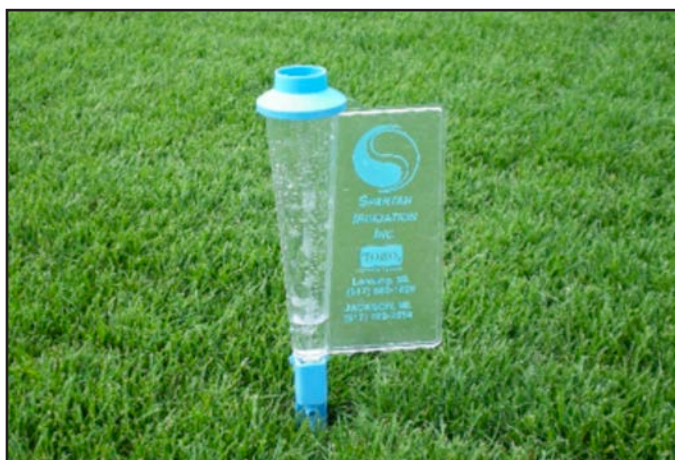
Image 4: Use a rain gauge (left) or collection cup (right) to determine your irrigation depth. Adjust run time to apply 0.25" per application 4 times per week to provide a cumulative weekly depth of 1". Photos provided by Alec Kowalewski.
