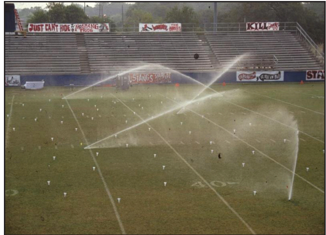
Irrigation Audit – Photo courtesy of Jeff Gilbert
