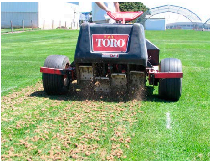
Figure 3. Hollow-tine aerification temporarily disrupts the soil surface, but it is one of the best things you can do for the health and performance of your field.
