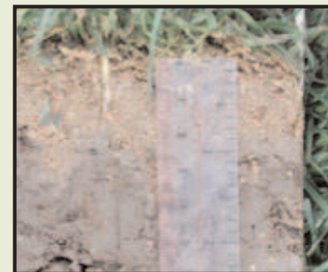
August 2007. Four sand-based topdressing applications applied to a newly established turfgrass stand over a one month period at ¼ inch per application, providing a 1 inch of sand-based root zone material, research plots at the Hancock Turfgrass Research Center, East Lansing Mich.,
